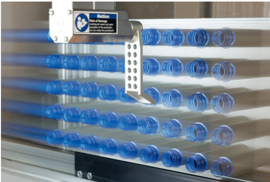
The ColorWatcher Integrated is implemented directly into the production machine, inspecting preforms immediately after they are produced.
