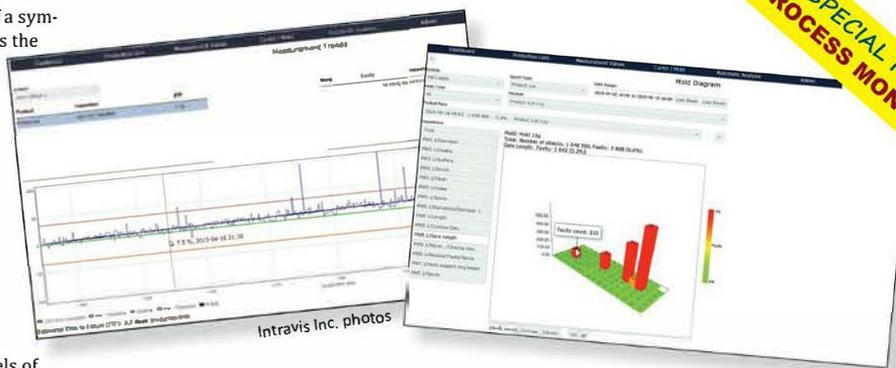
**Intravis' IntraVisualizer real-time production monitoring system is designed to convert production information derived from vision-based inspection into more usable data.**
