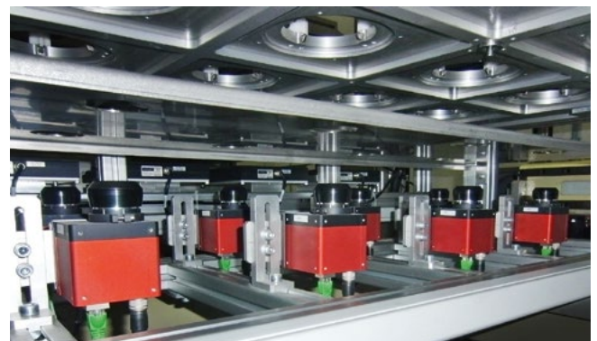
BarrierWatcher® integrated in the production line
