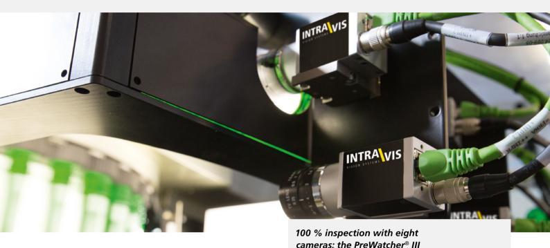
The PreWatcher® III inspects the quality characteristics of up to 72,000 preforms per hour with a **footprint of only eight square meters**. The orientation mechanism that operates with centrifugal force is integrated directly into the system.
